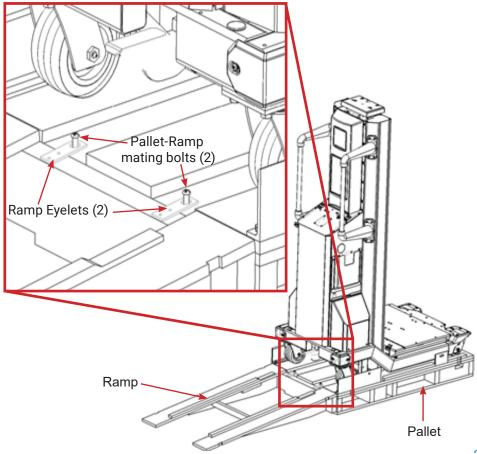
**Step 6:** Ensure brake is "off" per instructions in Operator's Manual. Holding both handles, carefully roll ServerLIFT unit down ramp to floor. Retain Pallet and Ramp for future shipping of ServerLIFT unit.
