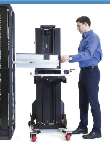
Getting servers in or out of slotted rails is awkward and tricky. The RS-500X Rail Lift safely tilts rack-mounted equipment to the perfect angle for aligning and guiding server nailheads into or out of J-shaped rail slots.
