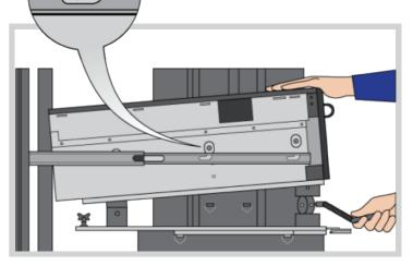
Once all nailheads are lined up in their respective rail slots, lower the ServerLIFT platform so equipment is fully supported by the rails. Reverse these steps for unracking server equipment.
