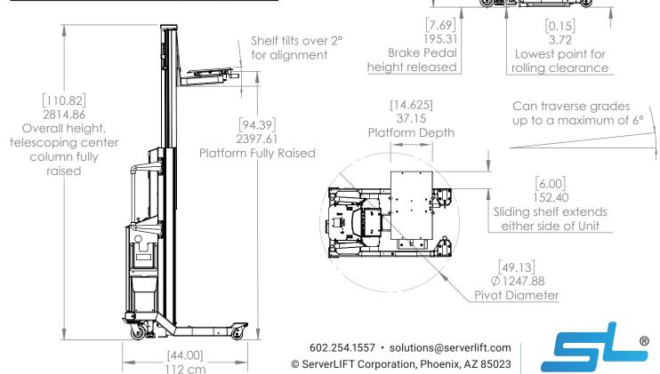
[52.95] 1345.01 Platform height, start of second lift stage (telescoping)
