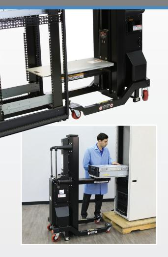
The ServerLIFT SL-500FX™ data center lift loads servers from the front with an extended shelf for deeper support into cabinets. This is especially useful when supporting servers for fixed rail and face-mounted installs. System integrators, test labs, or any facility with 5 ft (1.5 m) or more of space in front of the rack will benefit from its versatile, stable, and forward-sliding platform.
