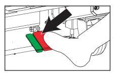
To engage Stabilizer Brake, depress red pedal until it locks in **DOWN** position. The back of the ServerLIFT unit should slightly lift up off the ground. The ServerLIFT unit should not move. If ServerLIFT unit moves, the Stabilizer Brake is not
