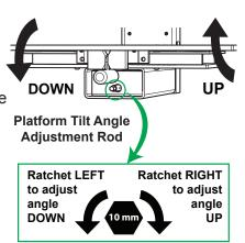
NEVER over-adjust the SmartTILT Platform angle. Adjust angle slowly and STOP as soon as resistance to the angle adjustment can be felt.
